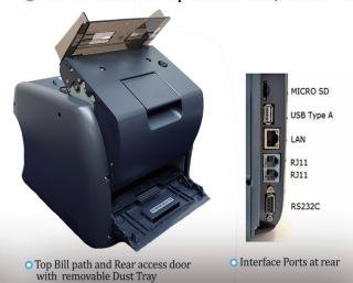
Complete Upper bill-path access from the top opening and Lower Bill-path access from Rear cover for easy and quick jam bill removal facilitate unique user-experience and smooth operation.
